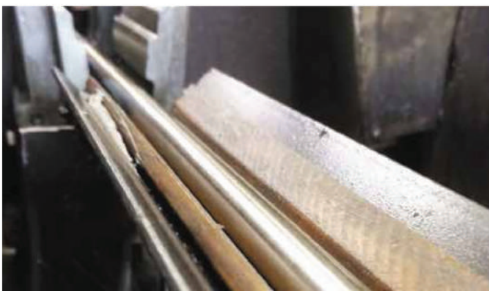
Through-feed centerless grinding for bar stock
