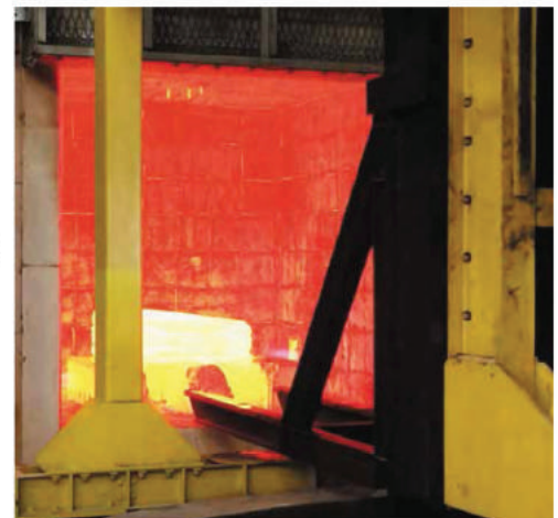
Batch annealing furnace
