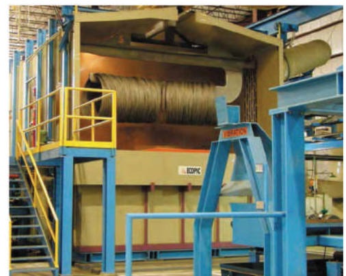
Acid pickling for oxide removal
