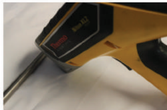
Grade verification via an X-ray fluorescence (XRF) analyzer. (PMI)
