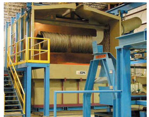
Acid pickling for oxide removal
