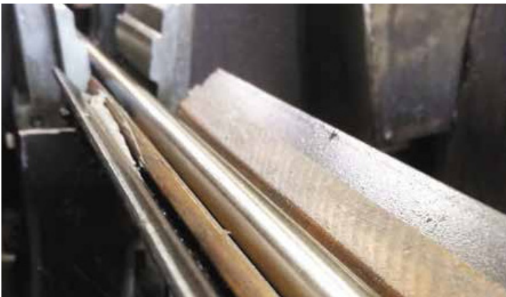
Through-feed centerless grinding for bar stock
