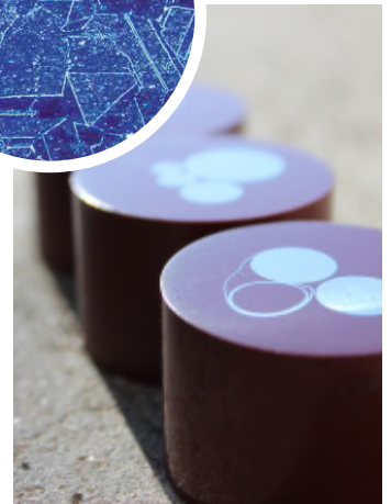
Material Sampling and polishing: product sample preparation for grain structure analysis and surface quality verification.
